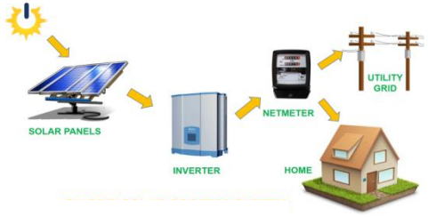
ON GRID SOLAR ROOFTOP SYSTEM
